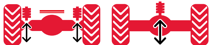
Independent suspension of both wheels
